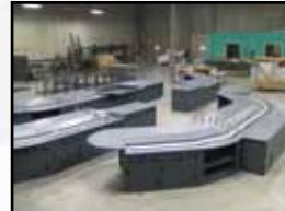
Consoles are dry fitted before being packaged to ship.
